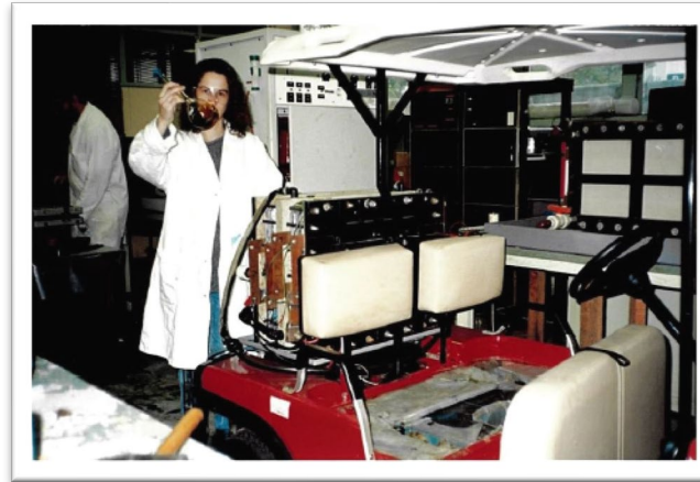
Glassy carbon electrode stack + 3 M vanadium electrolyte – R_{cell} = 2 \text{ ohm.cm}^2
